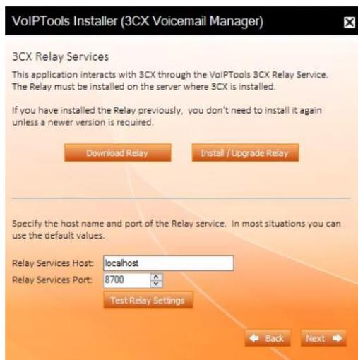
Figure 2: Test VoIPTools 3CX Relay settings
